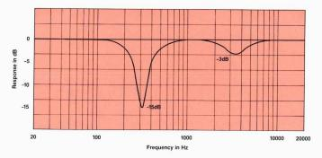
Combing Action of Filters at Typical E.O. Setting.
