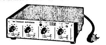
Experience with narrow band notch filters has demonstrated that in a typical single-microphone sound reinforcement system, gain before "howlback" can be significantly increased and intelligibility improved by centering a narrow band-reject filter on three or four of the most prominent system resonant frequencies. The Universal Audio 560 Feedback Suppressor provides an inexpensive, convenient, compact way to achieve this result.
