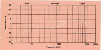
Frequency response contour of the 8120H taken in a hemispherical free-field environment. Measured response of a typical production unit, including all peaks and dips, does not deviate more than 4 dB from the above curve. Additional acoustic loading will further extend bass response.
