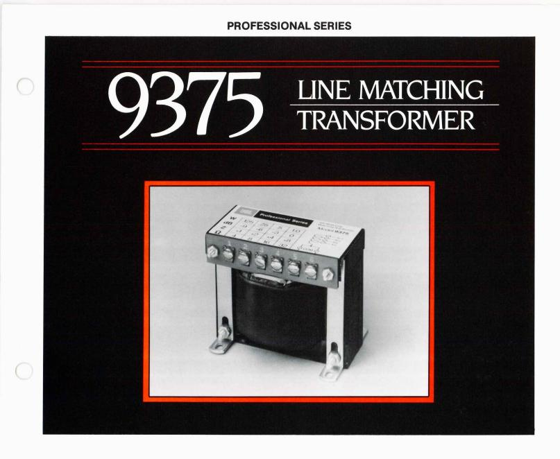
A 100-watt, wide-band autotransformer, the Model 9375 is designed for matching and balancing components in JBL professional speaker clusters. The 9375 allows matching 4  $\Omega$ , 8  $\Omega$ , 16  $\Omega$ , and 32  $\Omega$  loads in any combination; as an example, it may be used to match two 16  $\Omega$  high frequency drivers to a 16  $\Omega$  network. Frequency response is 30 Hz to 16 kHz,  $\pm$  0,  $\pm$ 1 dB, and total harmonic distortion is less than 1% in any configuration.
