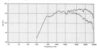
On-axis response, JBL 2385A, 1 W @ 1 m, dashed curved. With power response correction, solid curve.
