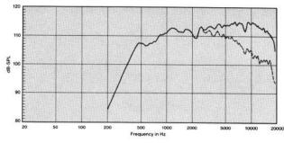
On-axis response, JBL 2385A, 1 W @ 1 m, dashed curved. With power response correction, solid curve.
