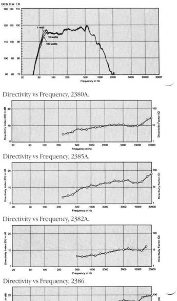
On-axis response, JBL 2380A, 1 W @ 1 m, dashed curve. With power response correction, solid curve.
