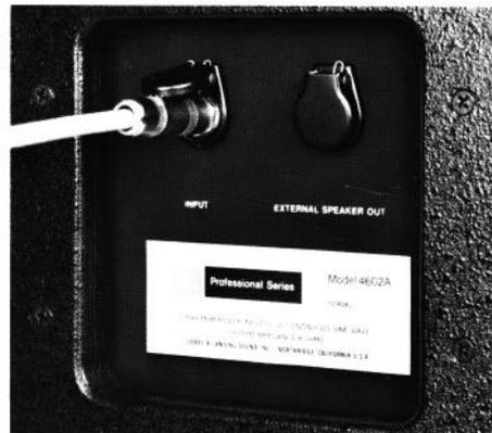
**Recessed Input Connectors.** Input and external output phone jacks are protected by spring-loaded covers to maintain acoustic integrity of enclosure. High current capacity telephone-type jacks provide positive high power connection.
