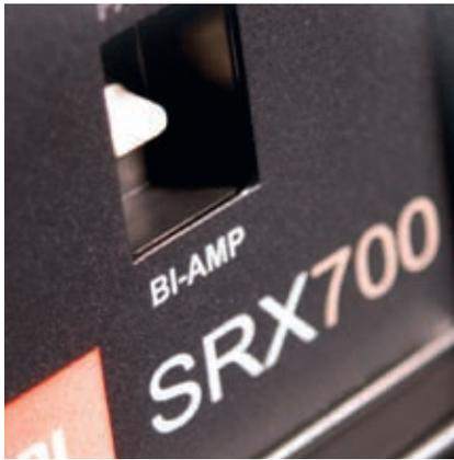
All SRX700 two and three-way models may be operated full-range or bi-amplified. The selection is made by means of a high-current, recessed switch mounted on the input plate. (SRX738 uses internal jumpers.) The same switch arrangement is used on the subwoofer to select  $\pm 1$  or  $\pm 2$  operation.
