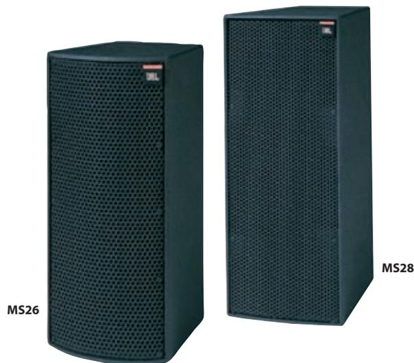
The Marquis Series is designed for use in fixed installation applications. This series has been value engineered to provide systems with the highest performance vs. cost available. The full range enclosures are pre-fitted with M10 threaded inserts and are supplied with an eyebolt kit. The MS26 and MS28 are equipped with "yoke mount" brackets and hardware. The cabinets suspend easily—both horizontally and vertically—offering a greater degree of versatility.
