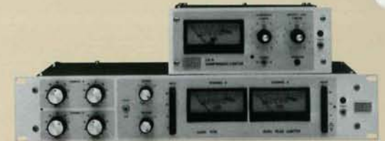
UREI MODEL LA-4 Compressor/Limiter RMS action, selectable compression ratios.
