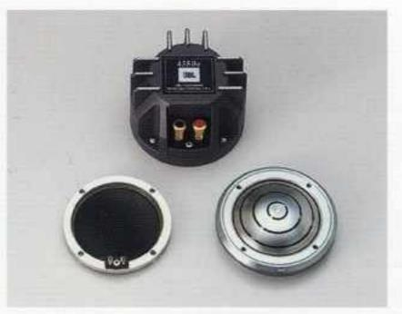
A die-cast-aluminum back cover with rib-type heat sinks provides a solid foundation for the superbly quick beryllium diaphragm and acts as a highly efficient heat radiator, permitting high-level output for extended periods of time. An extended back cavity is designed to handle frequencies below that of the crossover.
