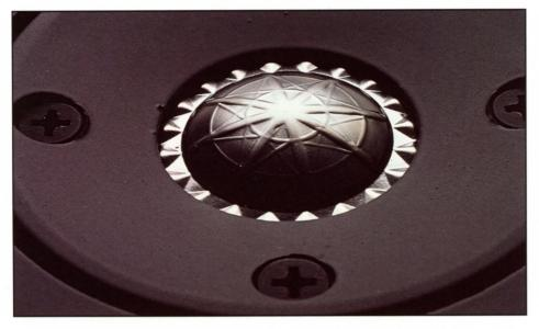
Titanium has an extremely high strength-to-weight ratio. But until recently, it could not be fabricated thin enough, light enough, to produce a dome. JBL solved that by developing a unique process that swirls compressed nitrogen gas against a film of titanium, only 25 microns thick thinner than a human hair. The process forms the dome perfectly and without causing stress fractures.
