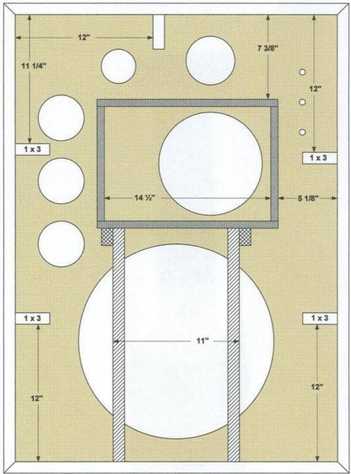
4345 BRACING DETAIL #2 - FRONT VIEW
