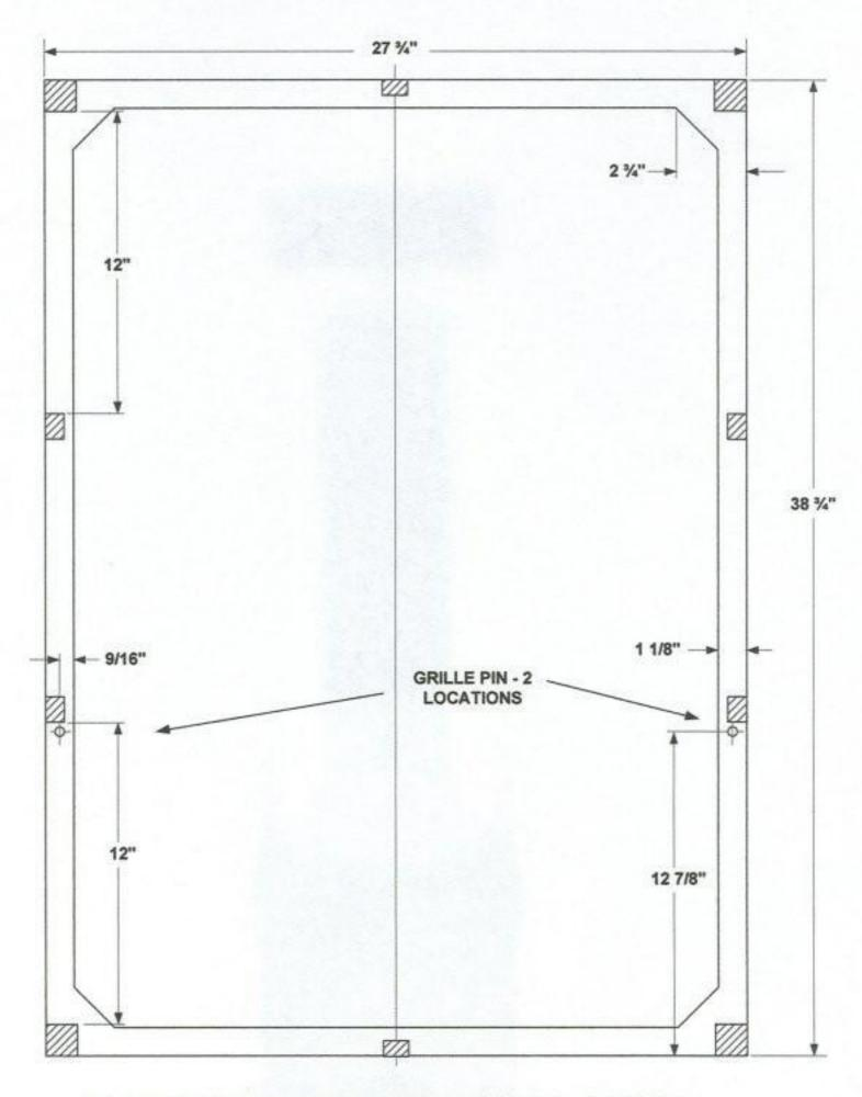
BASE FRAME IS 5/8" PARTICLE BOARD. CORNER AND SIDE STANDOFFS ARE PINE OR FIR.
