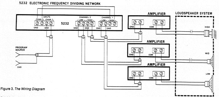
Shielded cable is necessary for all input and output connections, as shown. Make certain that the shield is properly connected to the ground terminal.
