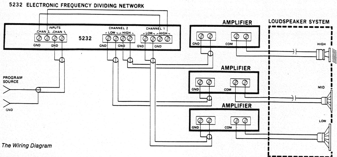
Figure 3. The Wiring Diagram
