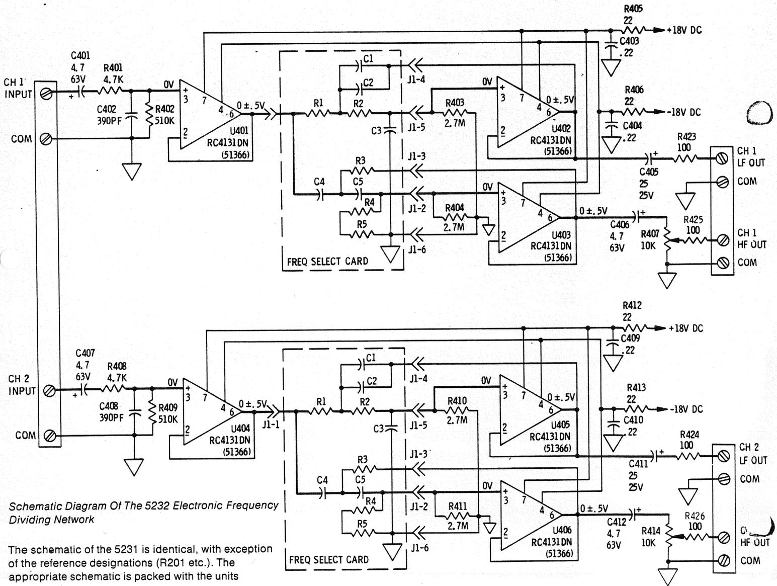
Schematic Diagram Of The 5232 Electronic Frequency Dividing Network
