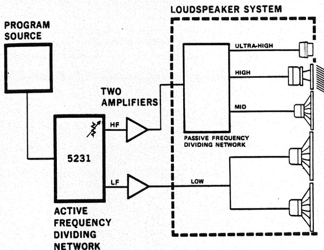
Figure 2. Combining Electronic And Passive Frequency Dividing Networks
