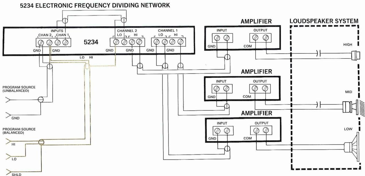
Figure 4. *Wiring Diagram For Tri-Amplification*
