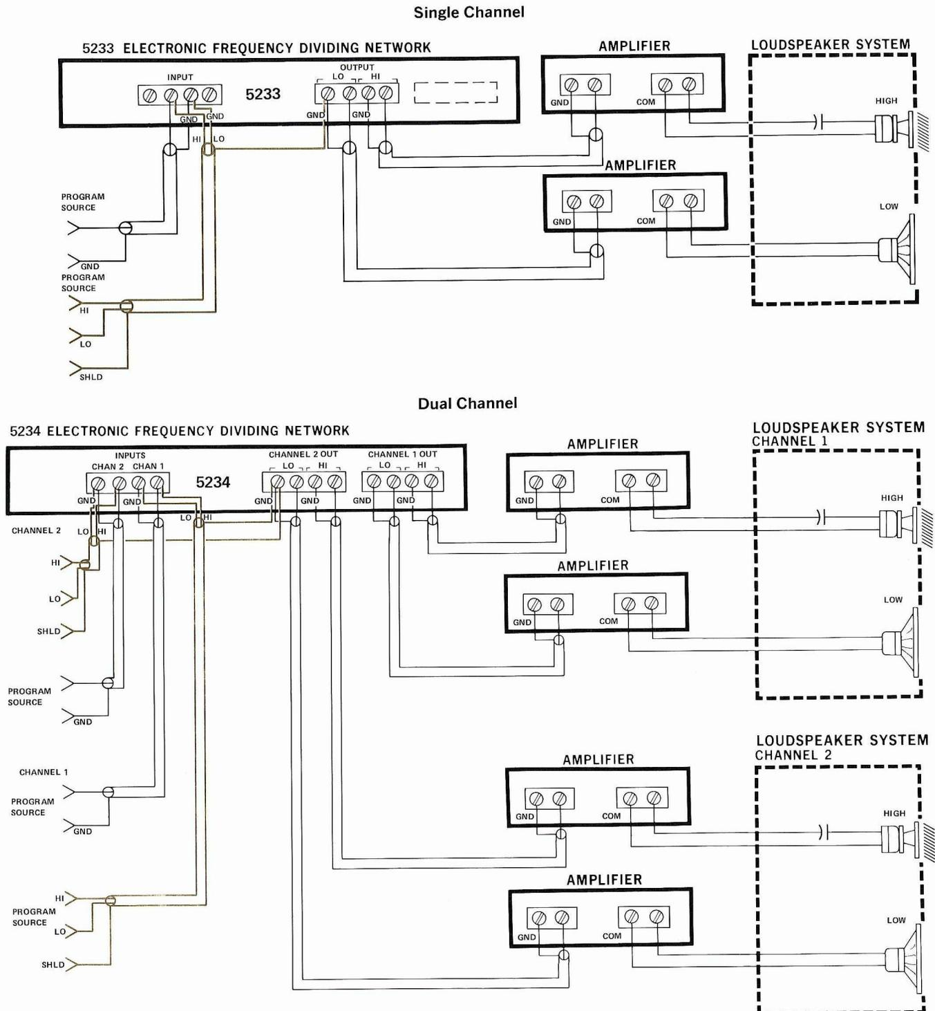
Figure 3. Wiring Diagram For Bi-Amplification.
