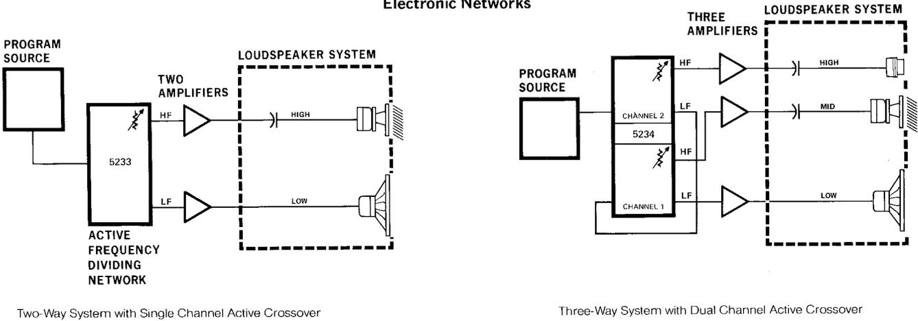
will drive the line inputs of conventional amplifiers. Two or more power amplifiers can be driven from each output.
