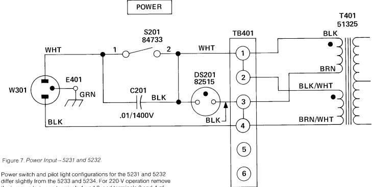
the jumpers between terminals 1 and 2, and terminals 3 and 4 of TB401, then connect a jumper between terminals 2 and 3.
