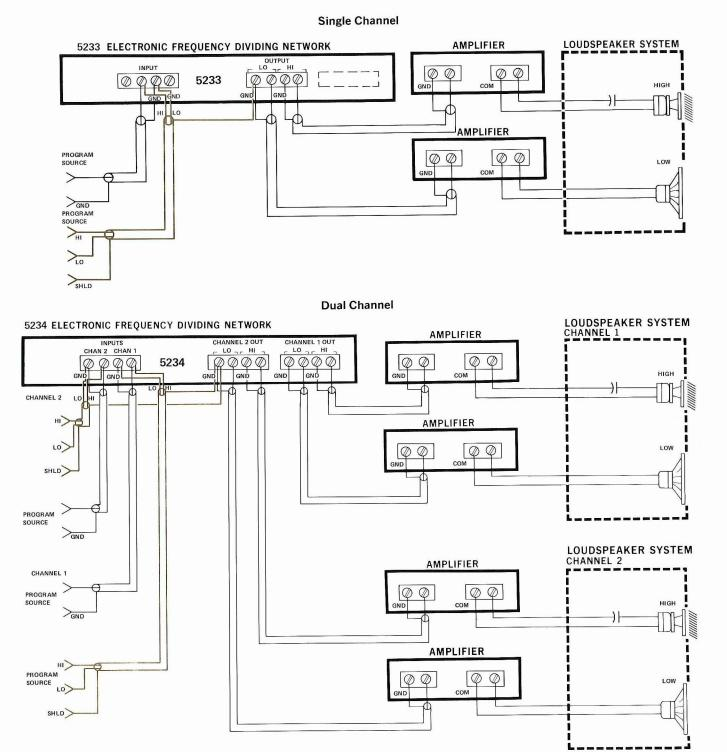
Figure 3. Wiring Diagram For Bi-Amplification.
