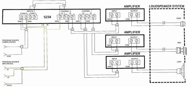
Figure 4. Wiring Diagram For Tri-Amplification
