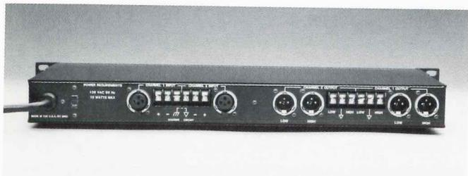
Input and output terminals for the 5235. The dual channels can be utilized for triamplification of a single loudspeaker system by connecting the low frequency output of one channel to the input terminals of the other channel. This allows separate, completely independent adjustment of the midrange and high frequencies.
