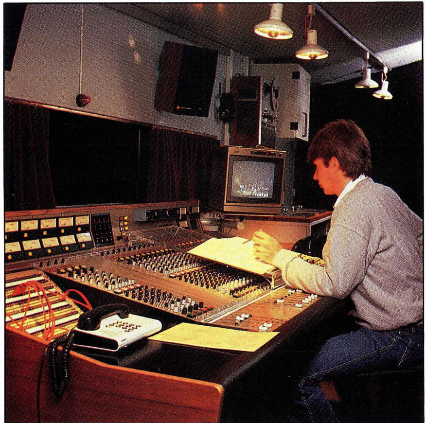
Two 4401 monitor loudspeakers are used in the control room because the first balcony blocks the clusters.
