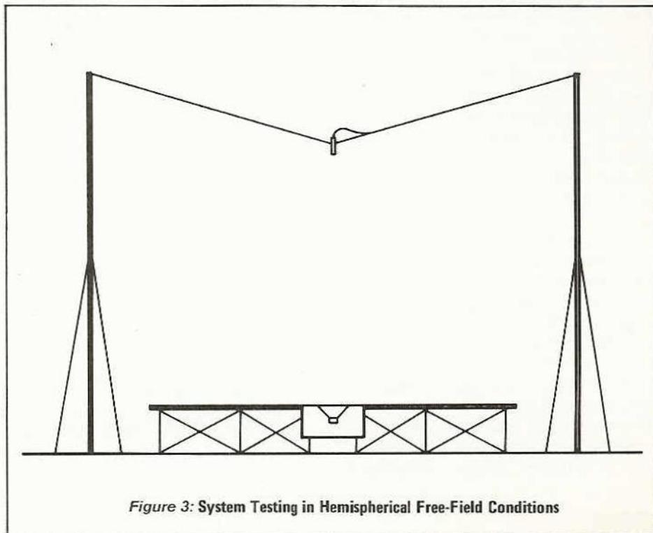
Figure 3: System Testing in Hemispherical Free-Field Conditions
