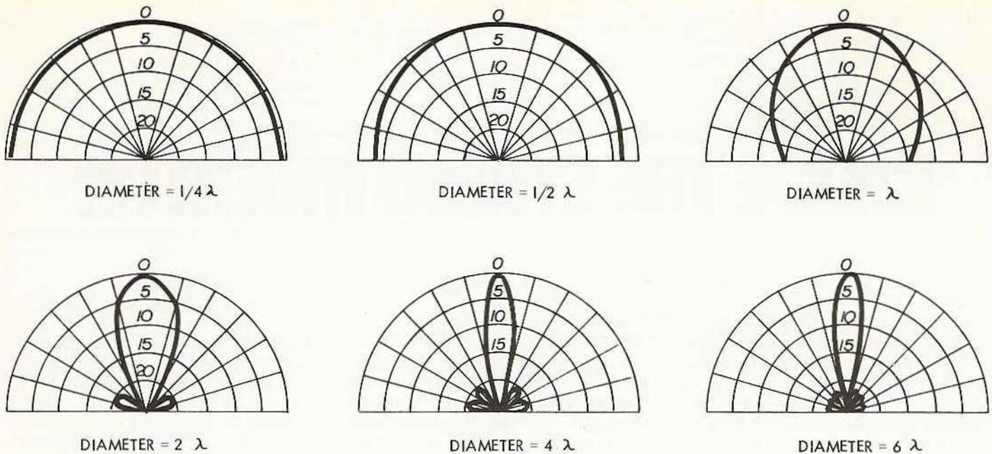
**Figure 2: Dispersion of a Single Direct Radiating Piston With Respect to the Wavelength of the Radiated Sound**
