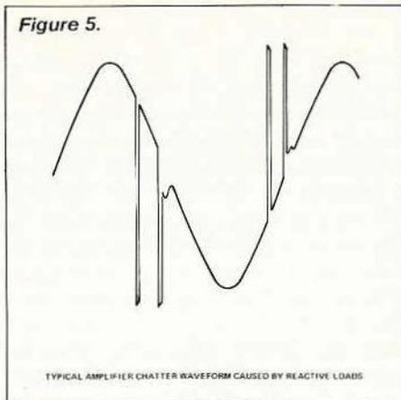
menon is much more likely to occur with reactive loads (such as those provided by large voice coils and massive magnetic assemblies) than with resistive loads, so it may not show up on a test bench. If chattering is a problem, increasing the available amplifier power or changing to an amplifier which does not exhibit chatter are recommended.
