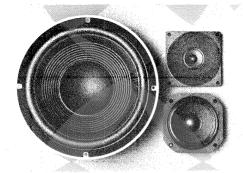
Loudspeaker System Components 10-inch Low Frequency Loudspeaker 5-inch Midrange Transducer 1.4-inch High Frequency Direct Radiator
