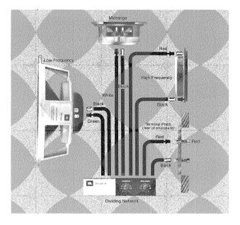
REPLACEMENT—Reverse the removal procedure to replace the loudspeaker system components. Mounting screws should be tightened evenly to avoid the possibility of frame warpage, and just enough to prevent air leaks between the components and the enclosure. Avoid excessive force.
