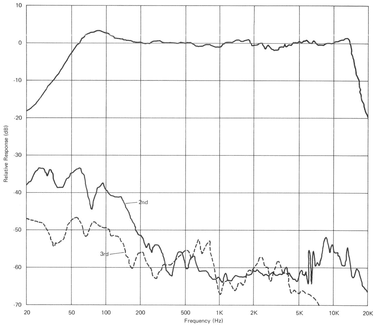
Figure 5 1W Harmonic Distortion
