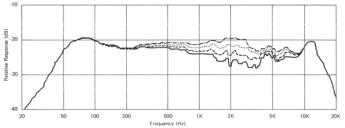
Figure 11 Mid-Frequency Control Action
