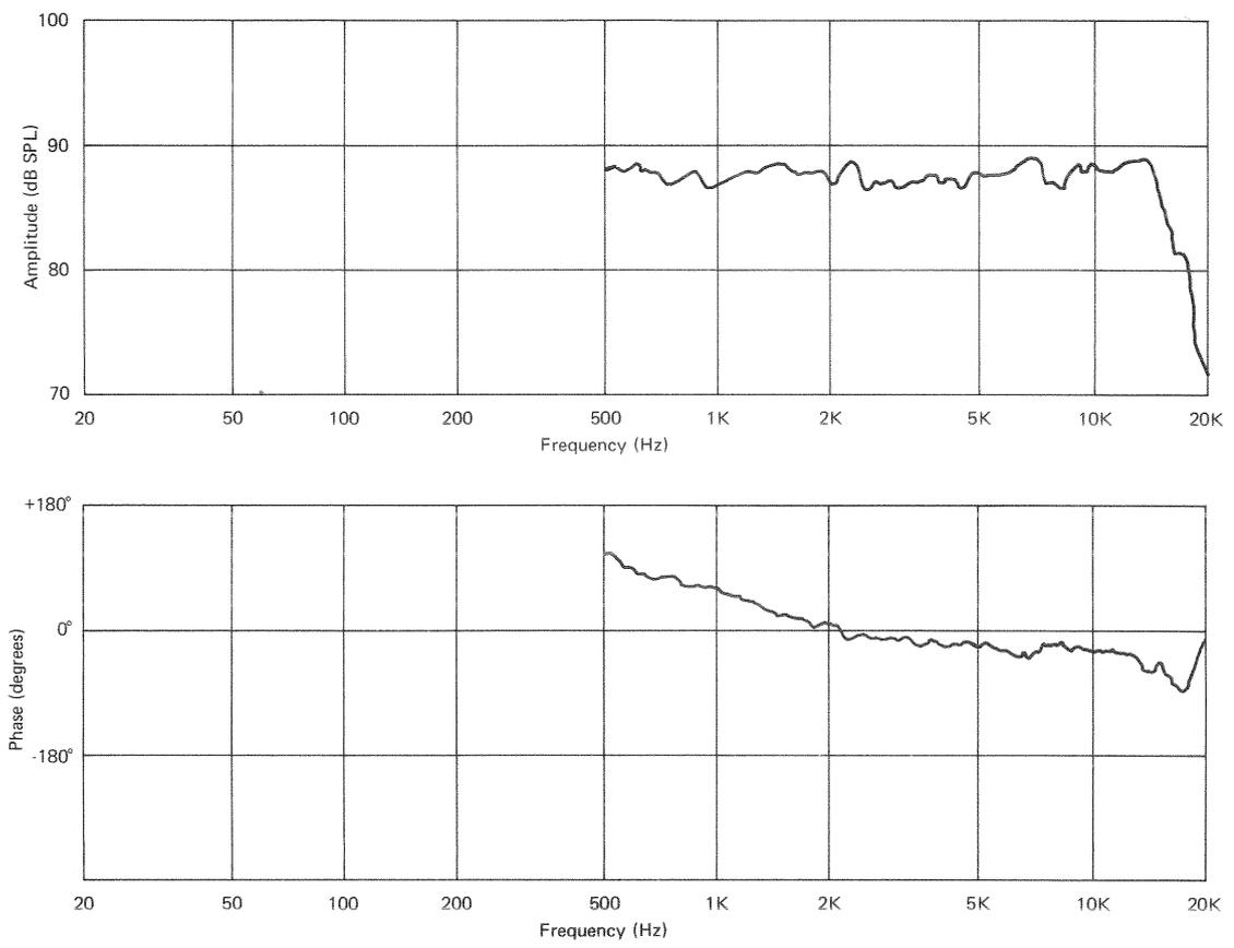
Figure 2 Anechoic Amplitude and Phase Response
