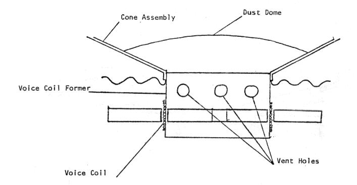
The cone used in the 127A was chosen as the result of research into many different materials, as was the choice of the dust dome size and mounting. Their specific choice, their mounting and interaction as a moving system, yields the smoothest, most extended response.
