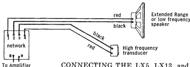
**CONNECTING THE LX5, LX13, and LX10.** These networks are connected to speakers as shown in the diagram below:
