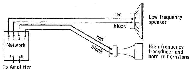
**CONNECTING THE N7000** The N7000 dividing network provides a means of adding the 075 to existing high-quality two-way loudspeaker systems to obtain added brilliance in the very high frequencies. It is connected to the high frequency terminals of the main dividing network as shown in the diagrams below:
