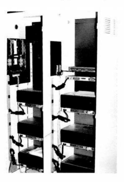
The 500-Hz high frequency output of the 5234 feeds one 6021 through a 600:600 transformer and a JBL 5195 input transformer. The output of this 6021 is connected to three 2482s in parallel, each with its own 20-µF protection capacitor. Two of the 2482s are mounted on JBL 2355 60-degree radial horns, and one is on a JBL 2350 90-degree radial horn. These horns are rated down to 500 Hz, making it necessary to restrict the bandwidth on these horns more than on the 2356s.
