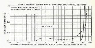
for brief periods of time. Prolonged operation with more than 40 watts output per channel will cut in the automatic protective devices.
