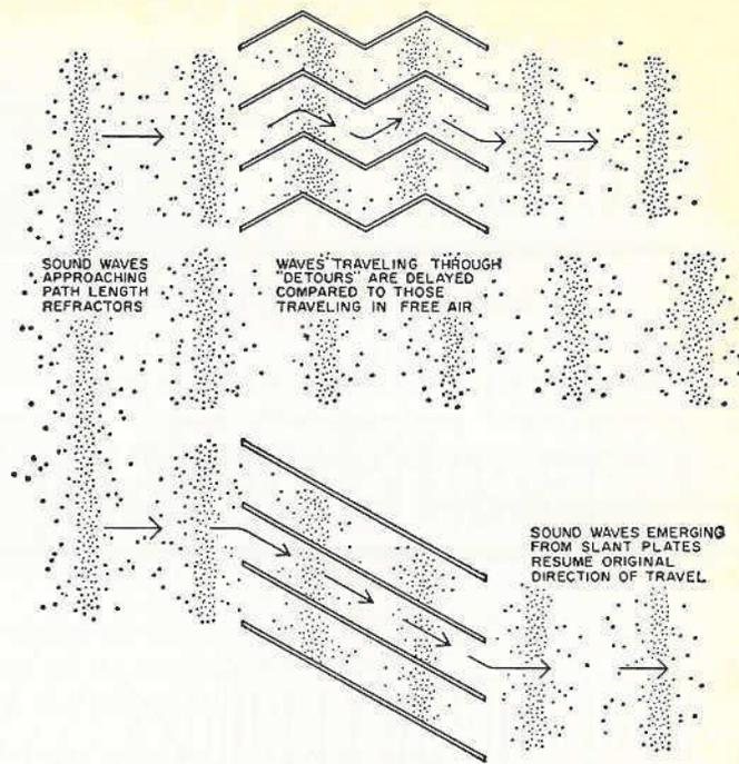
Fig. 4. Serpentine (top) and slant-plate path-length refractors.
