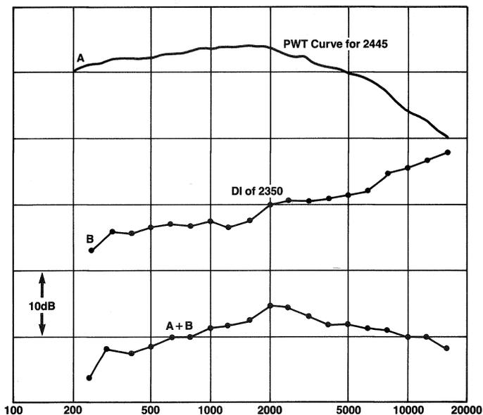
Figure 4 shows on- and off-axis curves for the 2445 driver mounted on the 2360 horn. In comparison with the 2350 horn, this model exhibits no beaming on axis. All of the on- and off-axis curves run fairly parallel with each other, and they all resemble the PWT response for the 2445 driver.
