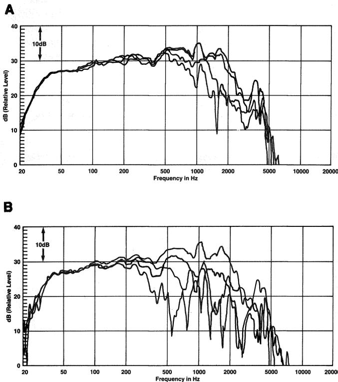
**Figure 8. Response, Horizontal (A) and Vertical (B), of 4550 at 0°, 15°, 30°, and 45°. (Dotted lines indicate ground plane equivalent low-frequency response.)**
