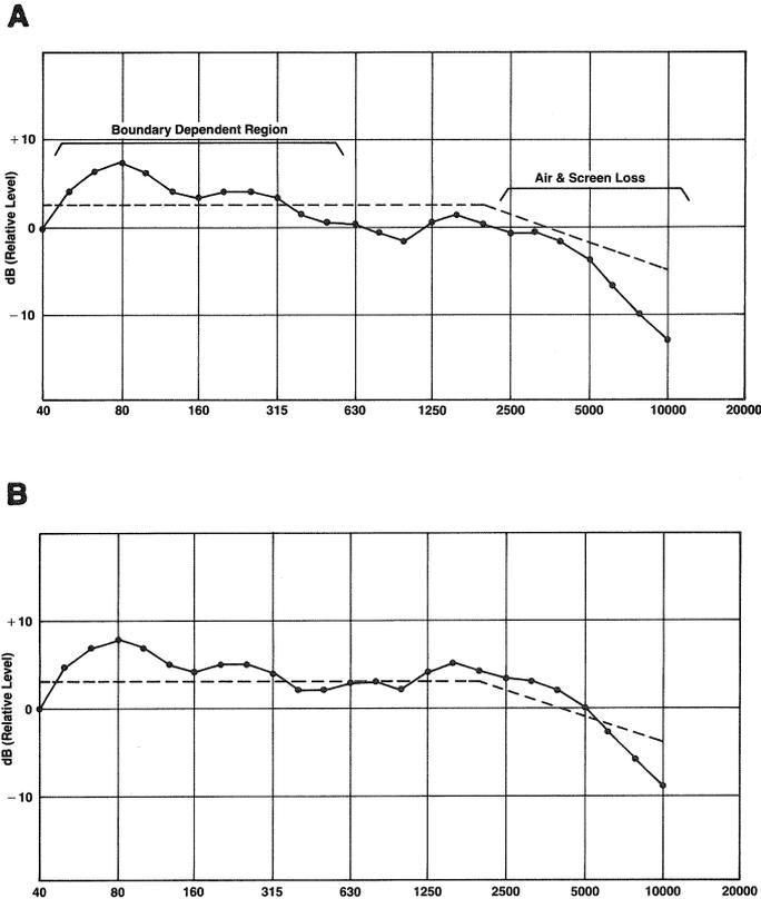
The degree of one-third octave equalization required to match the dashed line contour was quite small, as can be deduced from examining these curves.
