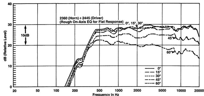
As one would suspect, the on-axis DI for the 2360 is relatively flat, as shown in Figure 6, and this indicates that there is no HF narrowing except for frequencies well beyond 10 kHz.
