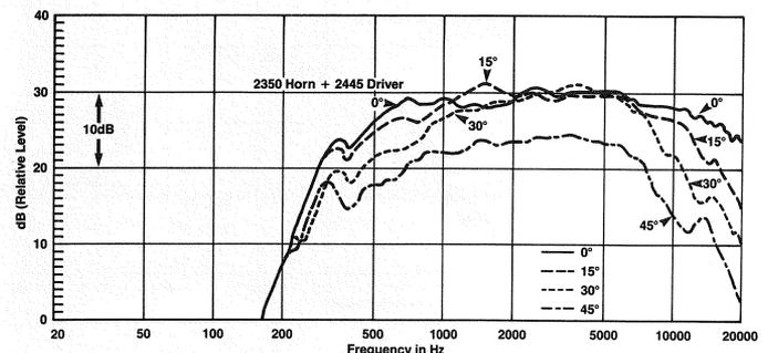
The horn "beams" on axis, and the degree of beaming is virtually the sum of the PWT curve for the driver and the on-axis Directivity Index (DI) of the horn. The DI of a horn may be thought of as the on-axis "gain" in dB, rela-
