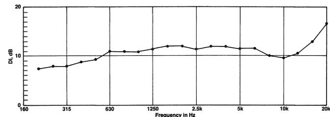
In general, a system with a relatively smooth on-axis DI can be equalized for flat power output over a wide frequency range. A system which has a rising on-axis DI cannot be successfully equalized, because the on-axis response will tend to rise at high frequencies.
