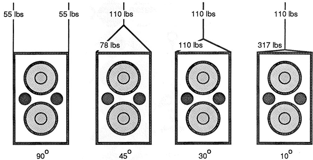
**Figure 6. Load Angle Efficiency**
