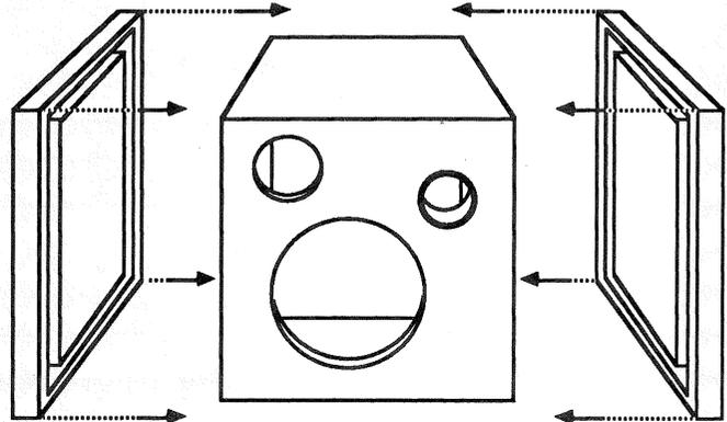
**Figure 14. Alternate Miter-Fold Construction**
