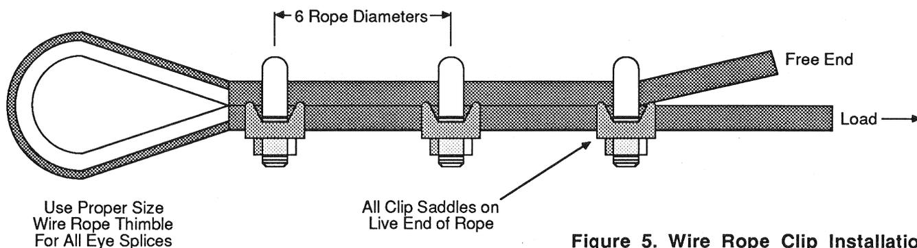
Figure 5. Wire Rope Clip Installation
