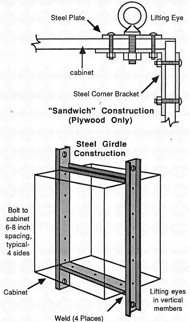
Figure 12. Cabinet Reinforcement
