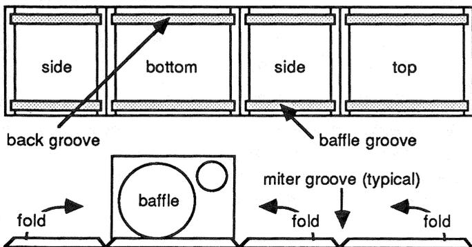
**Figure 13. Miter-Fold Construction**
