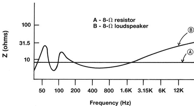
When we label Curve B as “8 ohms,” we are implying that the average load is somewhere around 8 ohms. At resonance peaks the value is considerably higher, while at some
