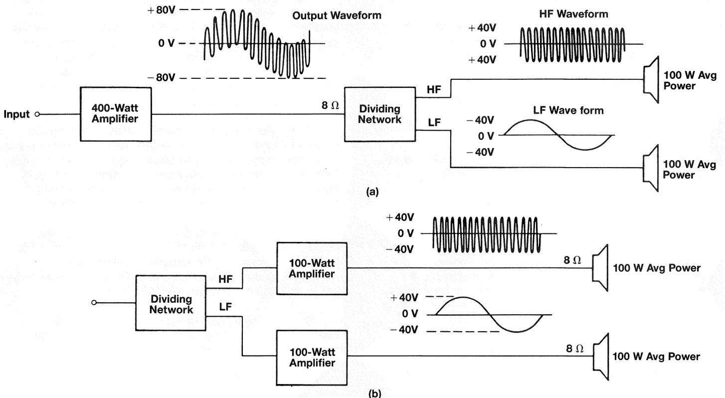
C. Use of highly stable amplifiers. (Some amplifiers recover from internal voltage clipping and current limiting less audibly than others. All else being equal, these are preferred for professional audio applications.)
