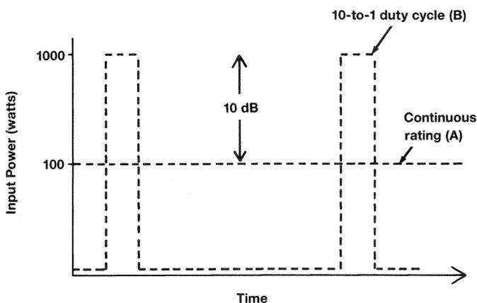
Most loudspeakers are capable of such operation — as long as the on-cycle is short enough that the voice coil temperature rise is insufficient to cause damage, and the off-cycle is long enough to ensure that sufficient cooling can take place. It is also essential that the bursts of input power be at a sufficiently high frequency so that the transducer is not mechanically stressed in the process.
