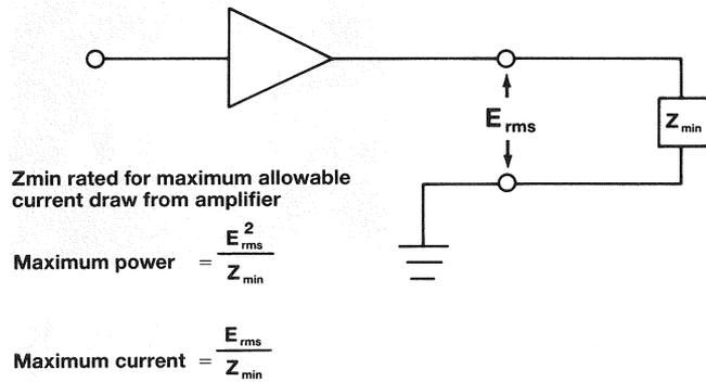
JBL and UREI have retained the traditional rating method for amplifiers, inasmuch as there is a wide universe of transducer hardware whose ratings are consistent with the older method. As an example, we will give the power output ratings of the JBL/UREI model 6290 stereo amplifier:
