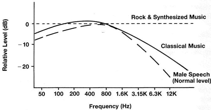
The designer must first determine the kind of spectrum to be reinforced. Then, calculations are made to determine average acoustical levels and the absolute peak requirements for headroom over these average requirements. Calculations may have to be made for several parts of the frequency range in order to cover all requirements.
