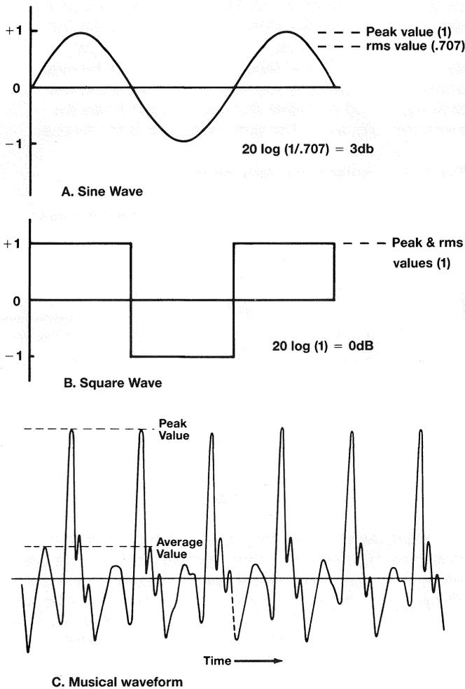
may have crest factors in excess of 10 dB, as shown in Figure 4C. Full band audio signals usually have fairly high crest factors, while bi- or tri-amplified signals, due to frequency division and consequent narrower bandwidth signals, generally have lower crest factors.
