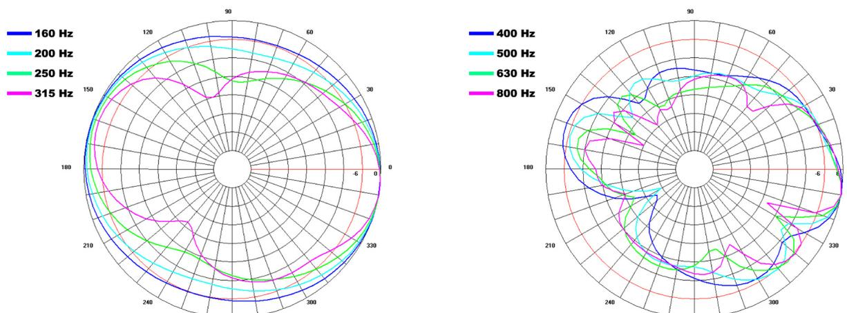
Fig. 8: Horizontally configured PD5322 - modeled vertical polar response
