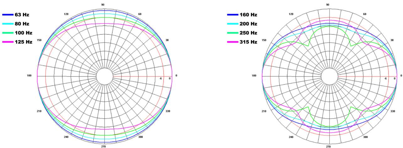
**Fig. 10: PD5122 shaded array - modeled vertical polar response**
