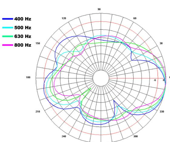
**Fig. 3: PD5322 + PD5122 - modeled vertical polar response**
