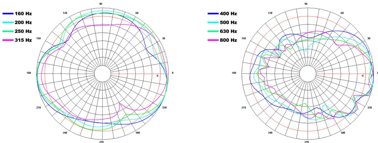
**Fig. 6: Vertically configured PD5322 - modeled vertical polar response**
