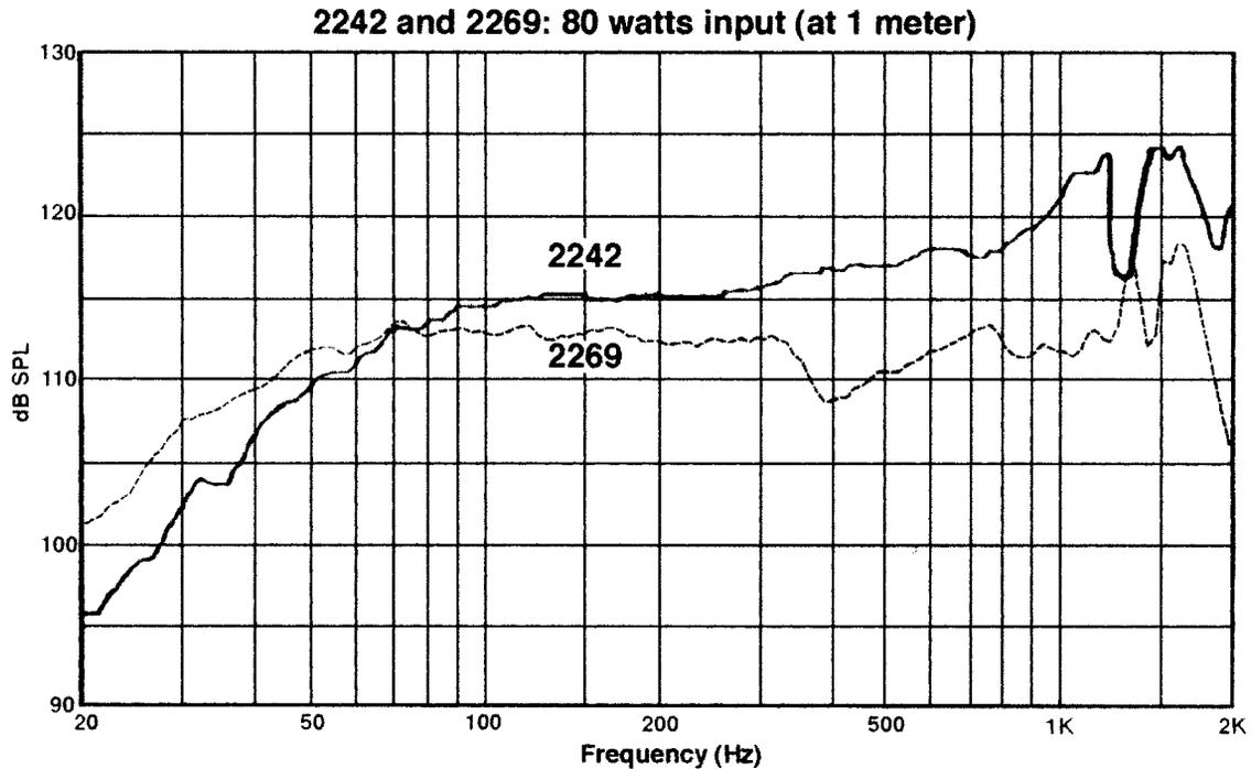
Figure 2. A comparison of on-axis output of JBL 2242H and 2269 drivers at 80 watts input.
