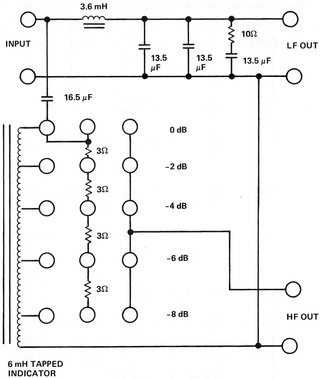
**FIGURE 1. SCHEMATIC OF UNMODIFIED JBL 3152A NETWORK**
