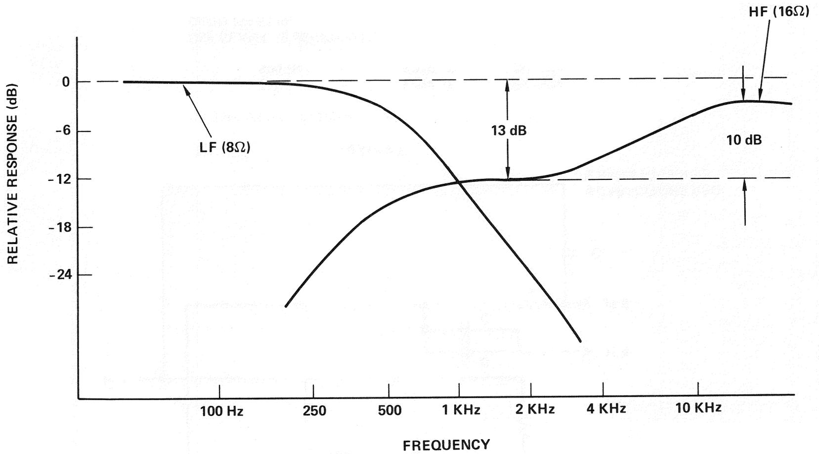
**FIGURE 3. RESPONSE OF MODIFIED 3152A NETWORK**
