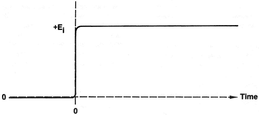
**B. Output of Band Limited, Non-slewing Amplifier**
