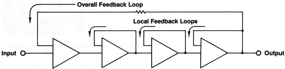
At the other end of the scale, there is the design approach shown in Figure 2. Here, local feedback around each stage reduces distortion as the signal is amplified, and moderate overall feedback is added just to stabilize gain and establish the DC operating point of the amplifier. The transit time problem is minimized, since the correction signal is fed around each stage. The JBL/UREI amplifiers are designed according to this philosophy.
