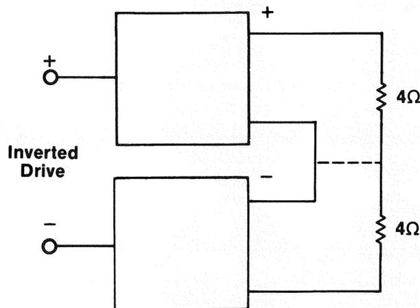
**Therefore,  $4\Omega$  rating applies to bridging with an  $8\Omega$  load**
