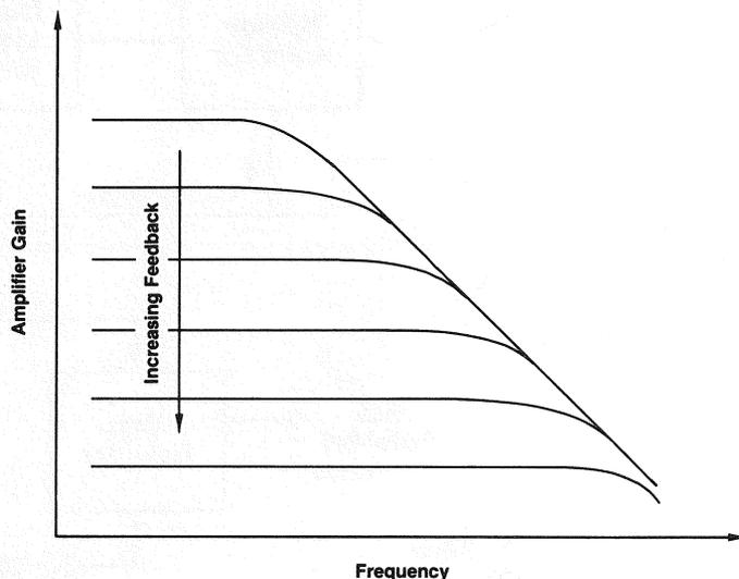
**Figure 2. Multiple Feedback Loops Within An Amplifier**
