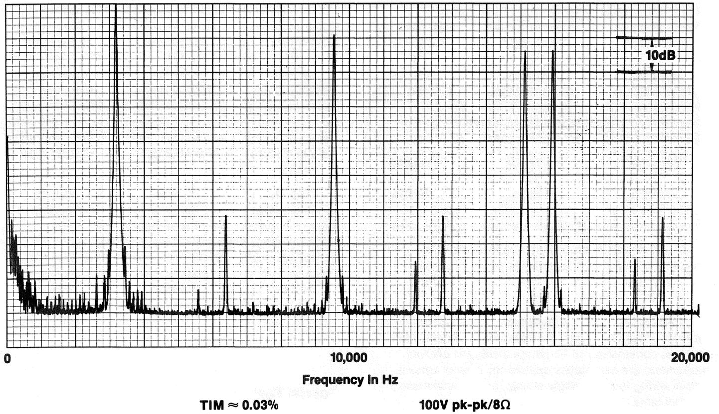
**Figure 6. TIM Spectrum, Industry Standard Amplifier using Quasi-complementary Circuitry**
