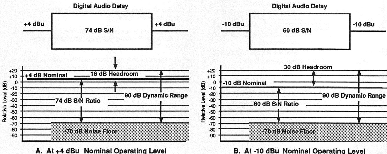
Figure 7. Headroom and S/N Performance in a Typical Digital Audio Delay.
