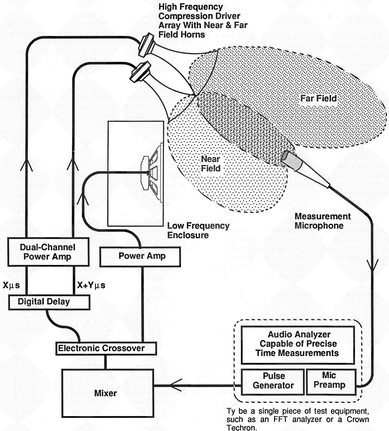
**Figure 5. Time Correction of An Array With Identical Drivers on Different Length Horns**
