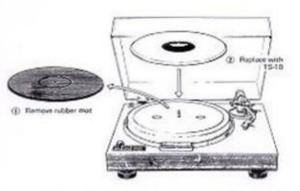
the material used for the platter mat. The TS-10 with its porous ceramic displays a short attenuation time and a low initial vibration when a single-pulse vibration is applied. In contrast, a rubber mat is hardly at all immune to low-range vibration, and with a glass mat, these vibrations are inherent.
