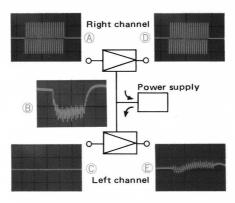
The disadvantage of a single power supply. A) A transient input signal is applied to the right channel. B) This signal affects the normally stable power voltage. C) The left channel has no input signal. D) The original input signal is amplified. E) When the same power supply (B) is used for both channels, a spurious 'ghost' signal appears in the left channel as an output signal. This is Dynamic Crosstalk Distortion. A dual power supply system successfully avoids this interference.
