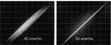
A synchroscope comparison showing the waveform of a bass drum as it appears through a conventional AC amplifier and a DC amplifier. The DC amp. displays no phase shift and appears as a clean straight line.
