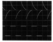
A 10Hz square wave oscilloscope comparison of AC (top) and DC (below) amplifier output signals. The DC amplifier shows no waveform deformantion.
