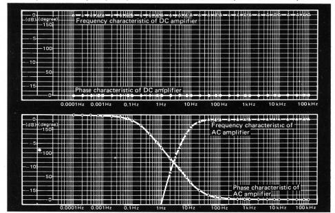
Only a DC amplifier's frequency response is completely flat from 0Hz to 100kHz.
