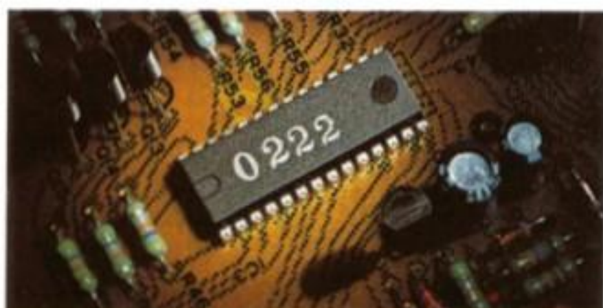
The "brain" that controls tonearm action.
