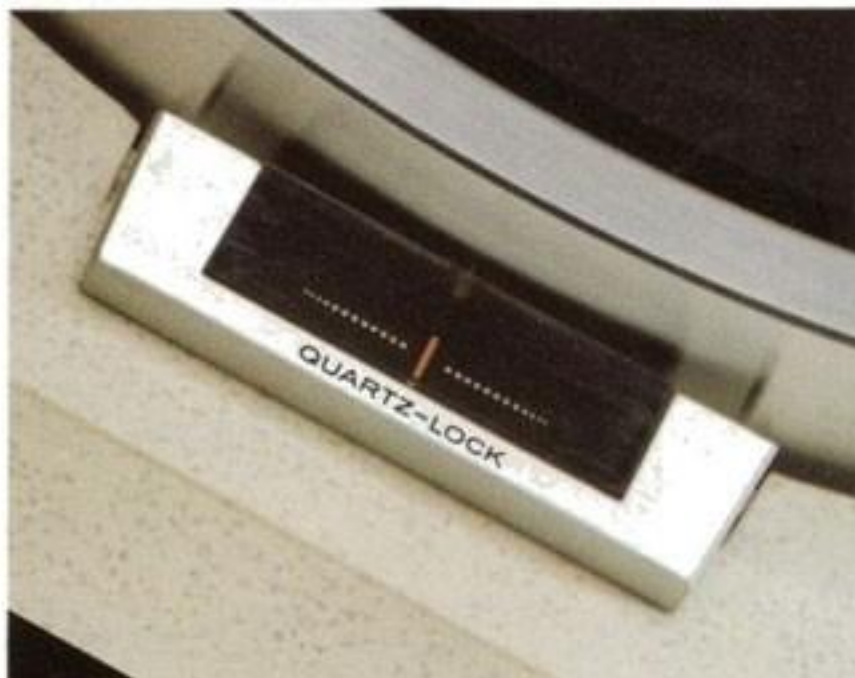
Quartz lock indicator lights up when PLL circuit is "locked" and turntable is operating at correct speed
