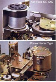
One way the KX-1060 prevents motor vibration from affecting the tape transport is the rugged, 12-rib rubber damper placed either side of the motor to "float" it.
