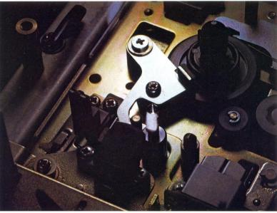
Special double back-tension system for the tape provides optimum frequency response in the 3-head design, keeping tape tension even and reducing frequency modulation effect.
