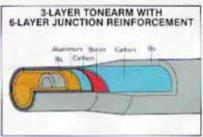
a tapered six-iayer structure is used. This careful design is largely responsible for the accuracy and clarity of reproduction across the audible range, particularly at low-level low frequencies that are most difficult to reproduce authentically.
