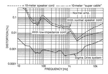
Above: the frequency vs distortion characteristics of a normal low amp into eight ohms, 20 Hz - 20 kHz. Measured at the amp. out
