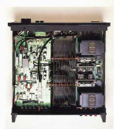
Interior of L-01A pre-main amplifier eliminates distortion with separate power sources via nonmagnetic body.
