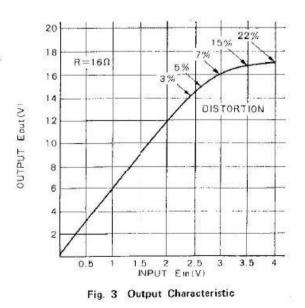
In case of the amplifier having the characteristic shown in Fig. 3, the maximum distortionless output may be calculated as
