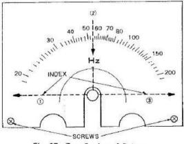
Fig. 17 Zero Setting of Pointer
