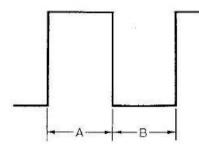
Fig. 16 Adjustment of Duty Ratio
