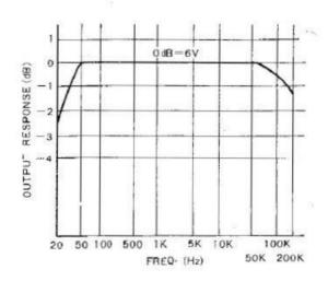
Fig. 4 Frequency Characteristic
