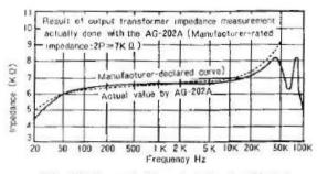
Fig. 11 Example Characteristic of a Market-Available Output Transformer
