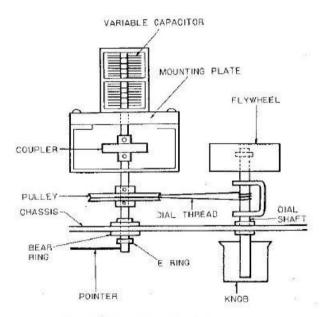
Fig. 15 The View of Dial Mechanism
