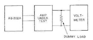
Fig. 2 Test Circuit
