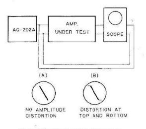
Fig. 7 Phase Characteristic Measurement
