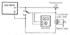
Fig. 10 Impedance Measurement
