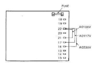
Fig. 18 Rewiring of Power Source Voltage
