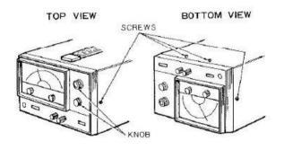
Fig. 14 Removal of Front Panel
