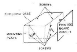
Fig. 13 Removal of Shielding Case
