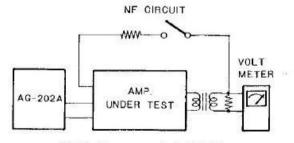
Fig. 6 Measurement of NF Value
