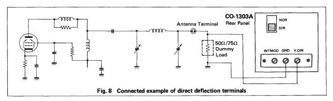
Remark: The dummy load should be of a non-inductive type as this may affect high frequency characteristics of the unit.
