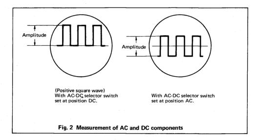
Any voltage measurements made on an oscilloscope are made in p-p or peak values. Because the effective, or rms value is often the one of interest, the following table gives the conversion between p-p and rms values for a number of common waveforms.
