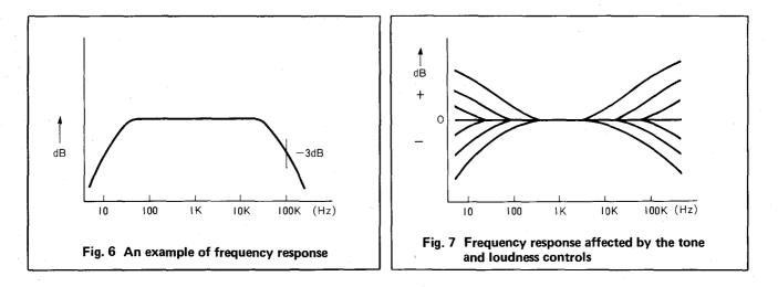
With the output voltage of the signal generator set at a constant value, change the output frequency of the generator and read the amplitude of the waveform in dB on the cathode ray tube screen using the dB scale for various major frequencies. Plot the amplitude readings thus obtained against the frequencies and you can obtain a general amplitude frequency characteristic as shown in the Fig. 6.
