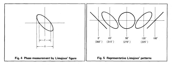
Note that if the EXT. GAIN control (12) is kept in the fully clockwise position in the above measurement, the vertical and horizontal signal phase difference of the oscilloscope is essencially zero up to about 2 kHz. Above 2 kHz, however, the unit will have a vertical and horizontal signal phase difference. Take the above fact into consideration when making phase difference measurements.
