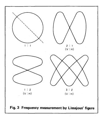
The frequency of signal oscillator and the unknown frequency are equal when the waveform becomes a straight line, an ellipse or circle. The figure comes to a standstill only when there is such relation between the frequency of the signal generator and the unknown frequency that the former is an exact multiple of the latter or vice versa. This makes it possible to find the unknown frequency through a calculation.
