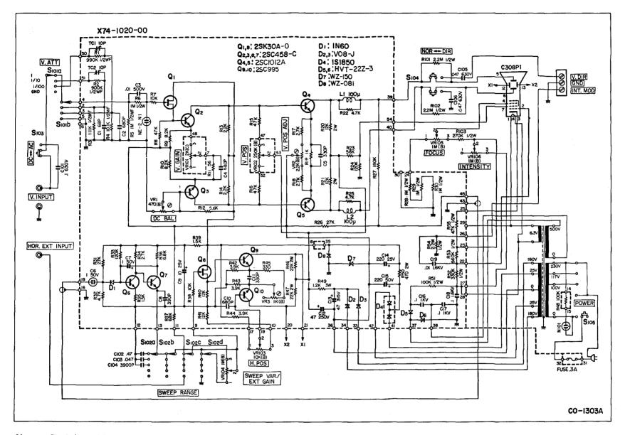
Note: Resistor with no specified value are those of 1/4 W and ±5%. Also, the circuit elements may be changed without notice owing to a technical innovation.
