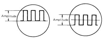
(Positive square wave) With AC-DC selector switch set at position DC. With AC-DC selector switch set at position AC.
