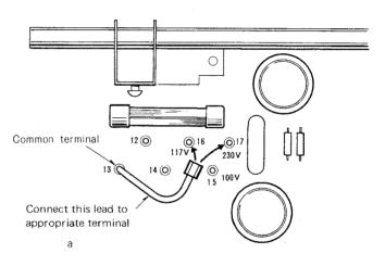
Fig. 13 Method of selecting power supply voltage
