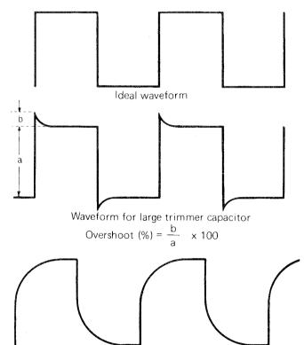
Waveform for small trimmer capacitor Vertical frequency response at high-frequencies (For example, it becomes 900k Hz, -3dB)
