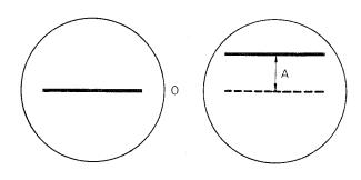
Sensitivity (V/cm) × A cm = Voltage (V) Fig. 3 DC voltage measurement
