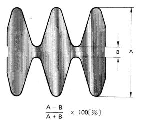
Fig. 12 How to measure modulation degree
