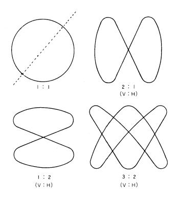
Fig. 4 Frequency measurement with Lissajous' figure
