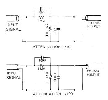
Fig. 7 Connection of attenuator
