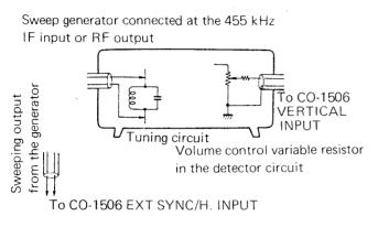
Fig. 11 Adjusting AM receiver
