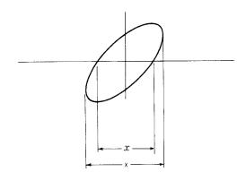
Fig. 5 Phase measurement with Lissajous' figure
