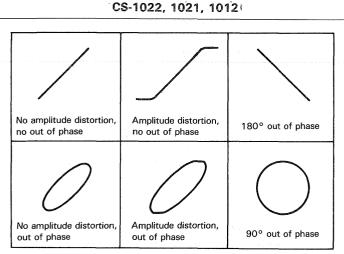
Fig. 26 Typical phase measurement oscilloscope displays
