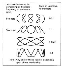
Fig. 27 Lissajous waveforms used for frequency measurement
