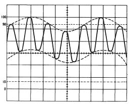
Signal containing undesired component (Broken lines: undesired component envelope)
