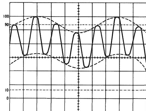
Signal containing undesired component
