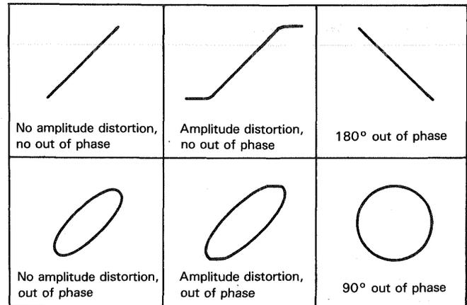
Fig. 26 Typical phase measurement oscilloscope displays
