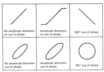
Fig. 26 Typical phase measurement oscilloscope displays
