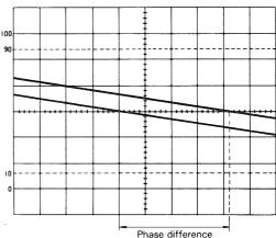
Expanded sweep waveform display.
