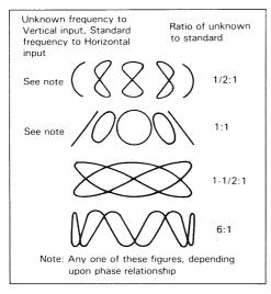
Fig. 27 Lissajous waveforms used for frequency measurement
