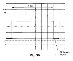
SWEEP TIME/DIV is 0.1 ms and apply 1.75 kHz reference signal. Adjust the SWEEP VARIABLE so that the distance of one cycle is 5 divisions.
