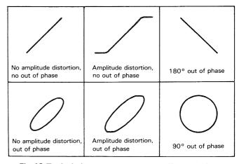
Fig.43 Typical phase measurement oscilloscope display
