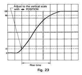
For the example, the horizontal distance is 4.0 divisions. The SWEEP TIME/DIV is 2  $\mu$ s. (See Fig. 23)
