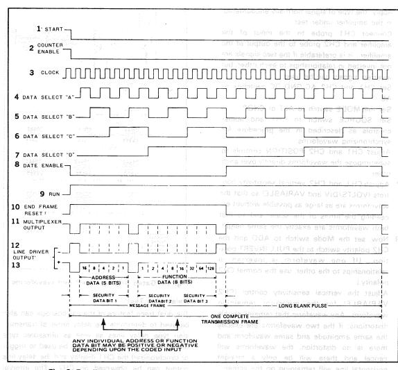
Fig. 9 Family of time-related waveforms from typical digital circuit in Fig. 8
