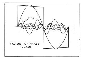
Fig. 33 Square wave tilt resulting from 3rd harmonic phase shift
