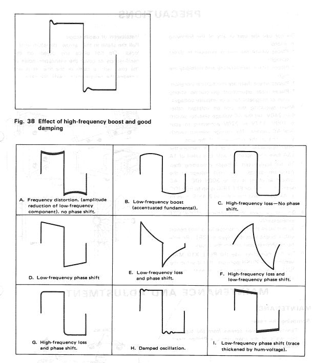
Fig: 39 Summary of waveform analysis for square wave testing of amplifiers
