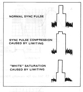
Fig. 22 Sync pulse waveforms
