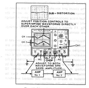
Fig. 10 Distortion measurement
