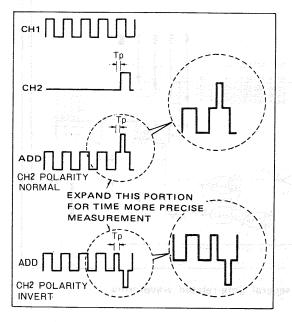
Fig. 7 Using ADD mode propagation time measurement
