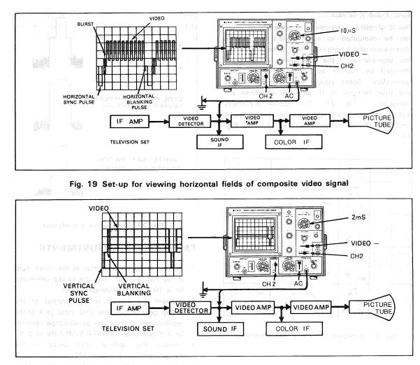
Fig. 20 Set-up for viewing vertical fields of composite video signal
