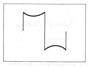
Fig. 32 Reduction of square wave fundamental frequency component in a tuned circuit
