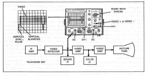
Fig. 18 Set-up for viewing fields 1 and 2 of VITS information
