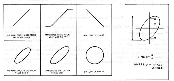
Fig. 25 Typical phase measurement oscilloscope displays
