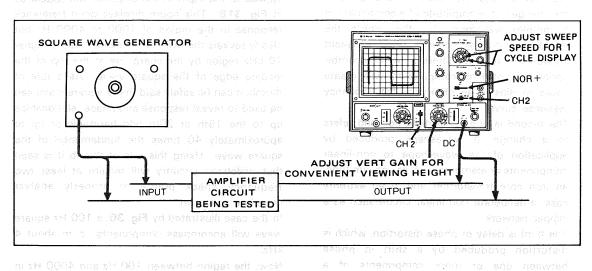
(101) vorces of the Fig. 28. Equipment, set-up for square wave testing of amplifiers of every weighted
