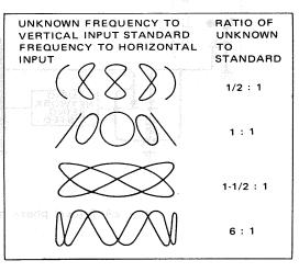
Fig. 27 Lissajous' waveforms used for frequency measurement
