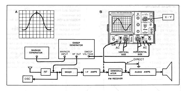
Fig. 23 Typical FM receiver alignment set-up
